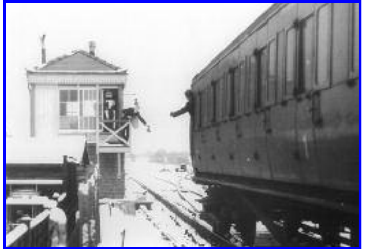
Driver Mick Stokes driving an Ascot to Guildford train about to collect the token for the single line at Frimley Junction from Signalman Jack Hills in the winter of 1968
